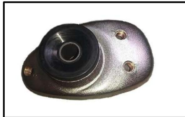
6. Press the bushing with hydraulic press to seat firmly in the metal housing:
