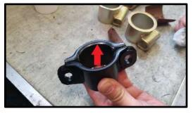
2. Clean and degrease all the sanded edge surfaces and degrease the silent bloc edges as shown:
