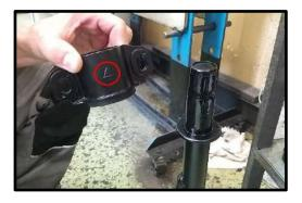
14. When the bushings with metal mounts are pressed on and the angle si right, leave A-arm in the press for approx. 5 minutes since the rubber bushing needs some time to seat propperly.
