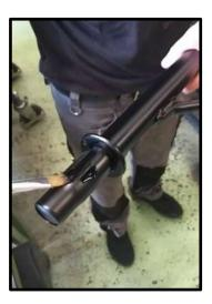
18. The angle of the front metal mount ears should be parallel with flat end of the U-shaped loop on the rear metal mount.
