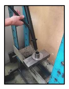
**12.** When pressing the metal mount on the A-arm make sure the angle between A-arm and the metal mount ear is 20 degrees.
