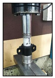
**6.** Once all the bushings are pressed in the metal mounts continue with pressing the metal mounts with bushings on the A-arm.
