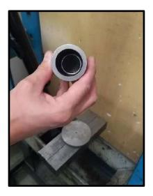
11. Use tool 2 from toolkit <u>PR98071P</u> from the upper side of the flange to press the metal mount with bushing onto the A-arm. Make sure to keep the right orientation of the metal mount – flange oriented downwards:
