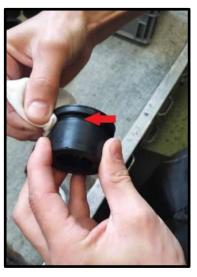
**3.** Lubricate the inner surfaces of both front and rear metal mounts (be careful not to lubricate the edge to be glued):
