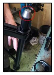
**9.** Lube tool 1 from <u>PR98071P</u> tool kit and the A-arm part where metal mount with bushing will be pressed on. Also lube the bushings inner surfaces:
