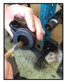
17. Make sure to keep the right orientation of the front metal mount. The arrow (marked with red circle) on the metal housing should point in driving direction:
