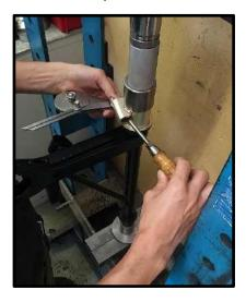
**15.** Lubricate the inner surface of the front bushing:
