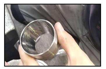
**6.** Be carefull to press the bushing into the bering flange in the right direction. Bushing has conical shape so installation orientation is very important:
