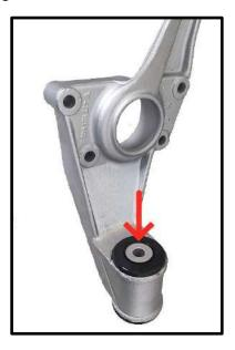
**3.** Once the bushing is out, clean the bearing flange. Optionaly you can sandblast it and repaint it. You can only renew undamaged (not cracked and not bent) bearing flanges, but usually there are light signs of corrosion to be found.
