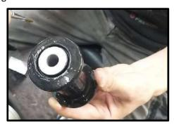
**5.** Lubricate the inner surface of tool 2:
