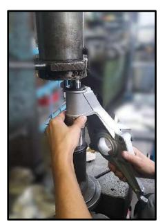
**8.** Check if both bushing edges sit nicely on the bearing flange housing edges and you are done:
